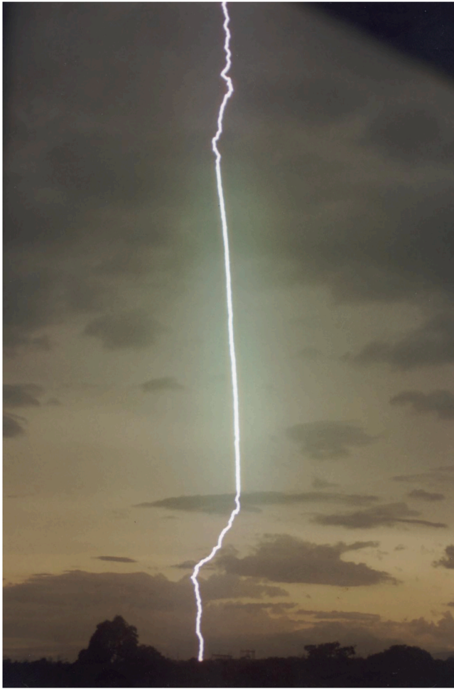
Fig. 9. Altitude triggered lightning (shot #3) strikes the ground at some 60 to 80 m from ESE-1; camera E.
