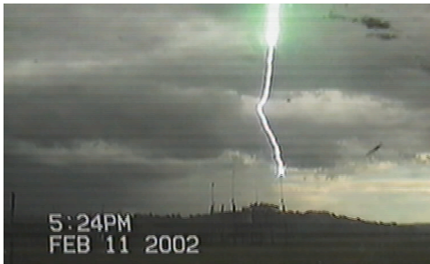
Fig. 4. Lightning strike to the Franklin rod (shot #33); altitude technique; camera B.
