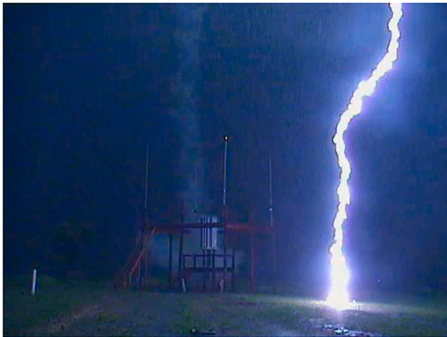
Fig. 8. Altitude triggered lightning (shot #0) strikes the ground at some 10 to 15 m from ESE-1; camera A.
