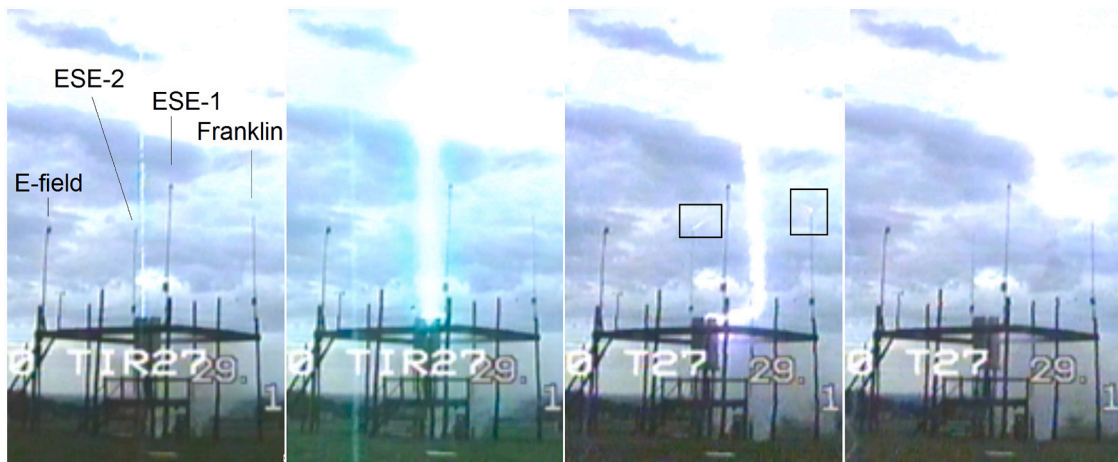
Fig. 11. Classical triggered lightning (shot #27); a) Wire burns with ICC; b) Subsequent return stroke; c) Another return stroke with channel apparently leaning to Franklin rod; d) Channel jumps to Franklin rod; camera B.
