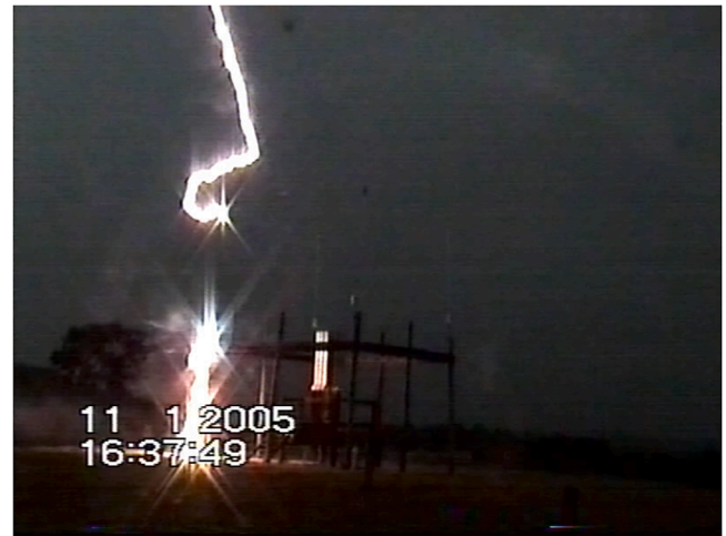
Fig. 5. Lightning strike to the electric field antenna (shot #51); altitude technique; camera A.
